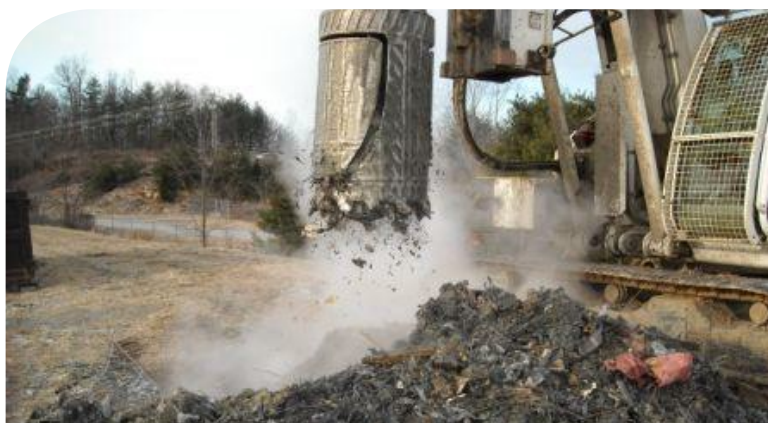
Figure 4.4: A bucket auger in operation
