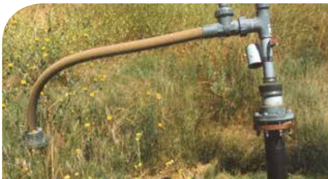
Figure 4.16: Relatively simple gas well head with sampling points and control valve, attached to conveyance system by reinforced flexible hose.
